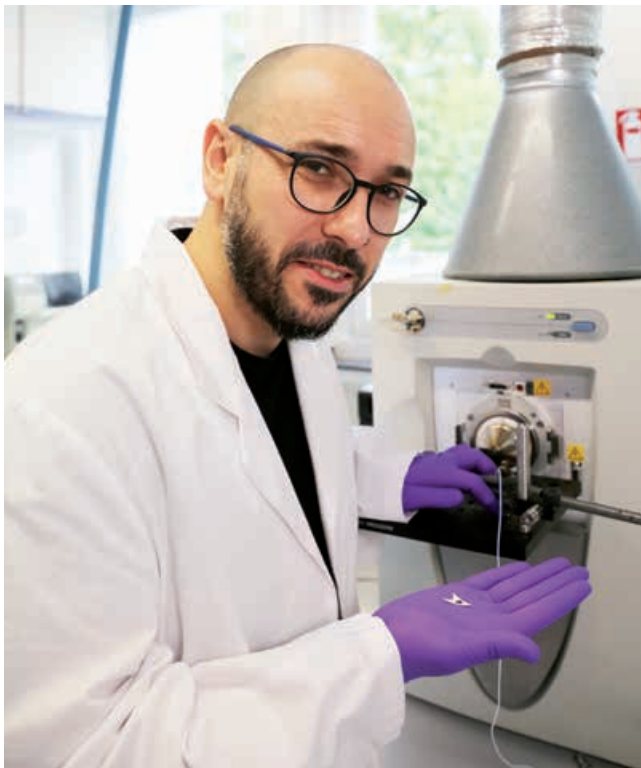
Using the mass spectrometer, Dr Marcos Bouza Areces examines animal blood samples directly on the filter paper for indications of a metabolic disorders.
