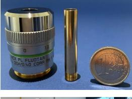
The diameter of a single ComplexEye lens (photo: centre) is 8 mm. It fits exactly under one 9 mm cavity of a standard 96 well pate. In a 384 well plate, cavities have a diameter of 4.5 mm. One ComplexEye lens is therefore many times more delicate and yet almost as capable as the 28.5-mm objective (left) of a conventional microscope. (UDE / Prof Dr Matthias Gunzer)
